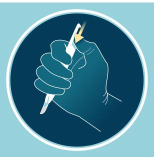
• Use thumb to deploy blade
