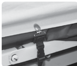
Fig. 3 - Sheet attachment clips (5750 only)
