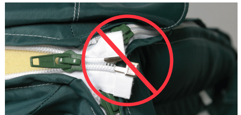
Zippers and zipper pins are not completely seated in their boxes and/or not all of the teeth are engaged.
