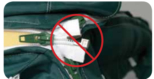
Zippers and zipper pins are not completely seated in their boxes and/ or not all of the teeth are engaged.
